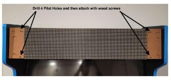
Note that Pixelcade should be flush with the bottom horizontal t-molding strip and extend .8" above the top t-molding strip.
