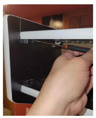
3. I suggest taking off the previously existing LED marquee strip lighting that is attached at the top of the cabinet, but it is up to you. I repurposed my LED lights by placing them on top of the marquee panel. There was a connection for the LED strip lighting at the corner of the marquee area which can be disconnected (and reconnected if you decide to repurpose this lighting as I did).
