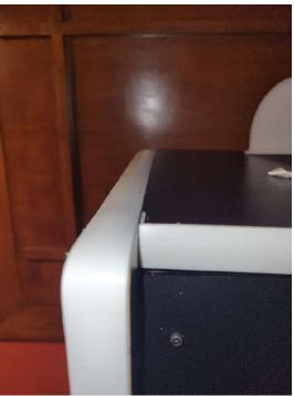
10. You will then attach your Pixelcade to the TAG cabinet. You should align the four holes in the corners of your Pixelcade to the four black brackets that are on your marquee panel. You can use the smaller wooden screws that come with your LCD Pixelcade. Again, I found it useful to drill a pilot hole first into the black bracket first before screwing in.
