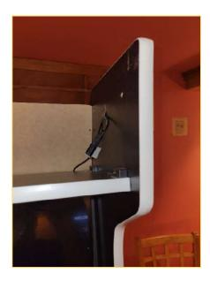
7. At this point or later, I recommend to cut out holes in your TAG back panel so that once your Pixelcade is installed you are able to reach the back of the Pixelcade's control panel in case you need to troubleshoot or decide to plug in a USB of your artwork. I'd do this before installing the Pixelcade to avoid dust on it. See below.
